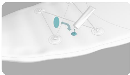
Apply one layer of glue on the patch and on the damaged area
