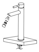
Remove the aerator and turn on faucet for 1-minute to flush debris from faucet and feed lines. Turn Faucet off and re-install aerator.
