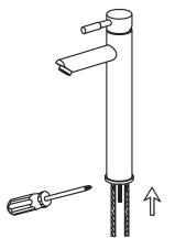
Secure the threaded mounting stud by inserting it into the hole in the tap body and tightening it with the screwdriver.
