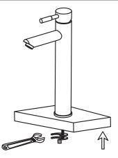
Place mounting hardware over mounting stud under sink. Secure with mounting nut. Tighten mounting nut securely.
